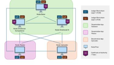
The ledger architecture is designed in two layers: Layer 2 (PoA) for document validation and Layer 1 (PoW) for securing the ledger. Both layers are interconnected through a single reference value (layer2\_block\_hash) stored in the PoW ledger, creating a strong linkage between them. This dual-layer design ensures that each transaction is represented in two different blocks, making the system more resilient against manipulation.
